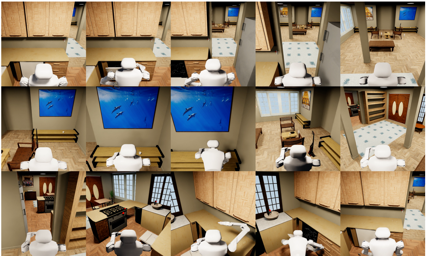
Fig. A.9: Successful task completion by a participant. The robot navigates to a dishwasher and opens it, moves to a table to collect teacups, returns to the dishwasher, places the teacups inside, and closes it.
